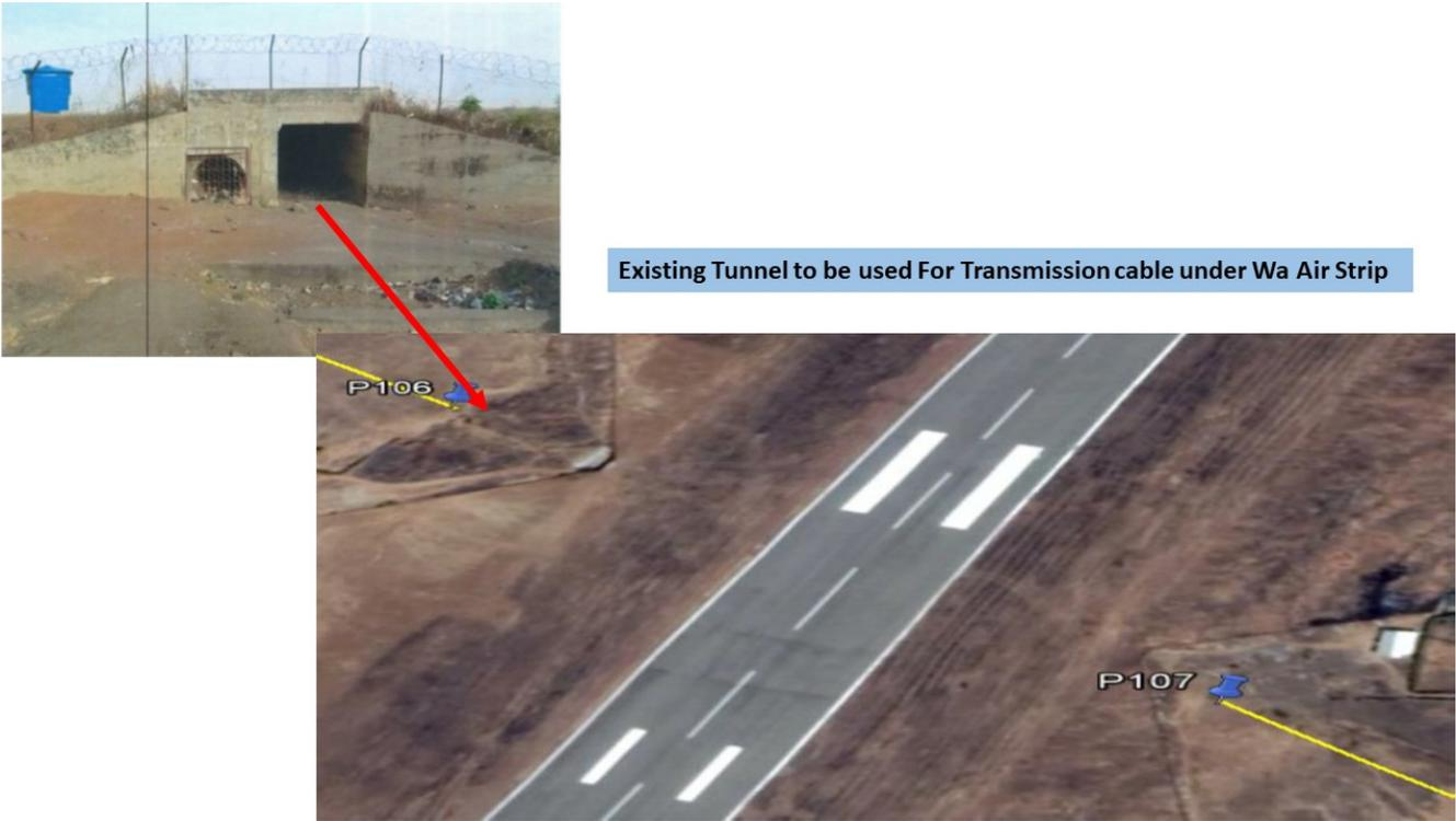
Plate 3-1: Area under Wa-Airstrip for underground interconnection line
